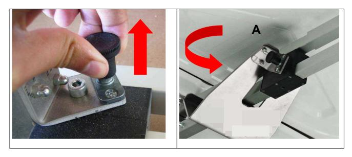
Release the back retainer by rotating knob (B). Rotate the knob anti-clockwise.
