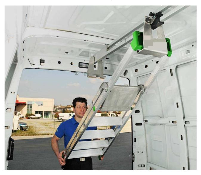
Lock the retainers in position by rotating knob (A) and (B) clockwise. Complete the securing of the step ladder by fastening the belts provided.
